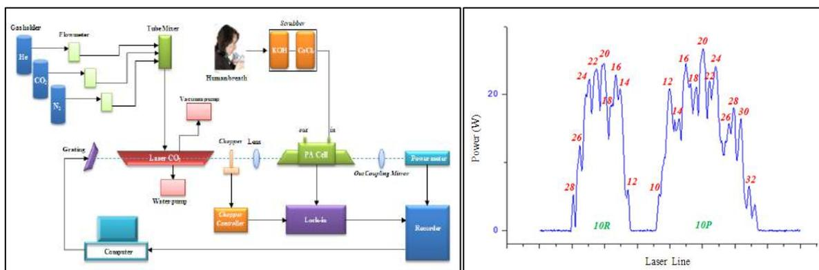
**Figure 1.** (a) Laser photoacoustic spectrometer, (b) The output spectrum of the laser power CO<sub>2</sub>.
